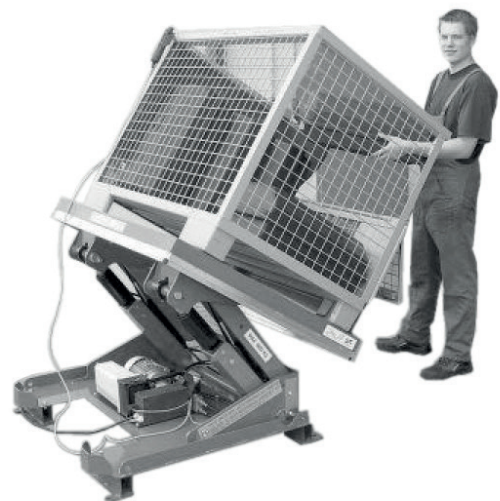
Item no. 2750004 Lifting and tilting of wire cages
