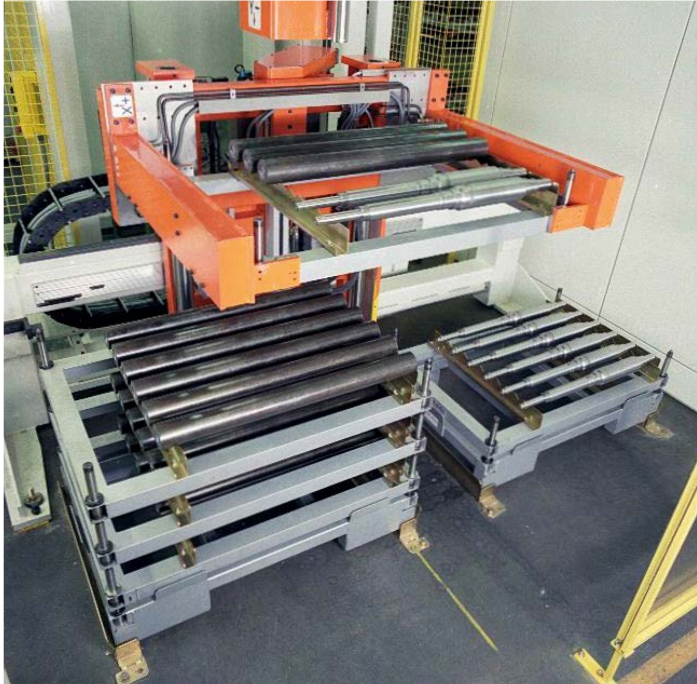
Workpiece carrier with a handling system for automated transport
